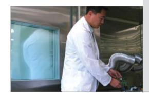
To ensure reliability, the HALT chamber combines powerful thermal and vibration technologies to test a product and its components beyond product specifications.
